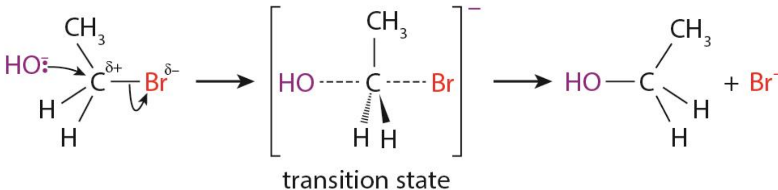
Figure 22.8: The S N 2 mechanism showing the transition state (activated complex).
